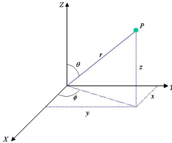
FIGURE 12. Spherical coordinates
